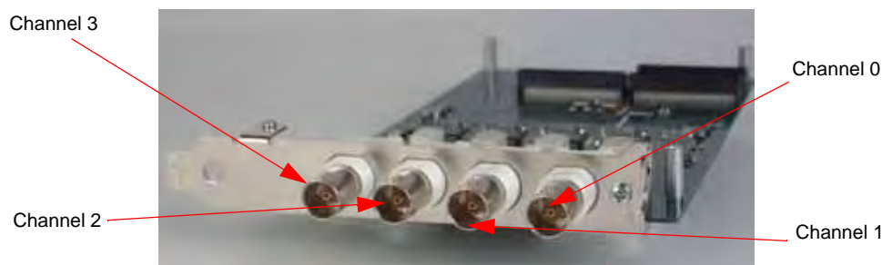
Figure 1. Connector Pinout, BNC
